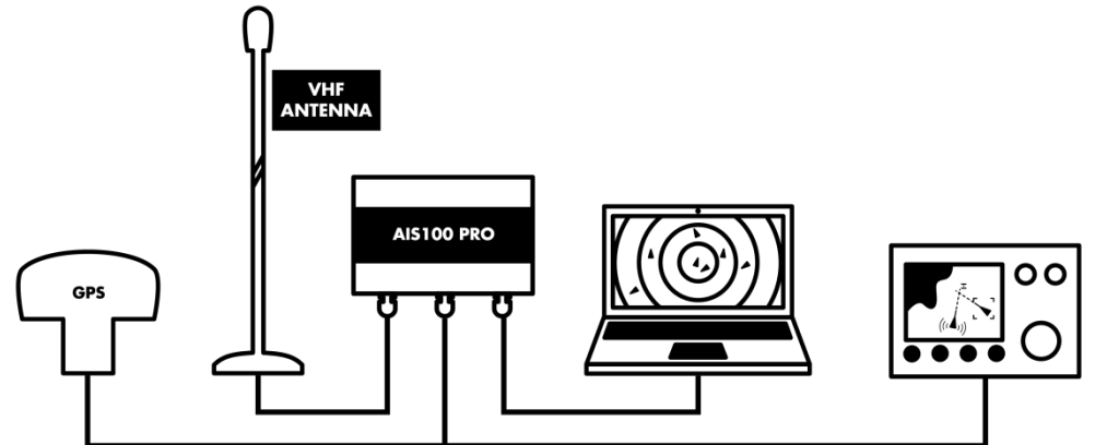
PC+Plotter AIS Receiver Installation
